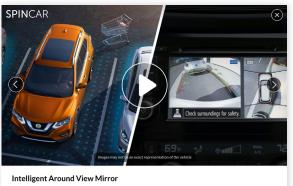
Creates a virtual composite 360-degree bird's-eye view of your vehicle and the area surrounding the vehicle and allows you to select front, rear and curbside split-screen views. Moving Object Detection can warn you about moving objects that come into view of the cameras with audio and visual alerts.
